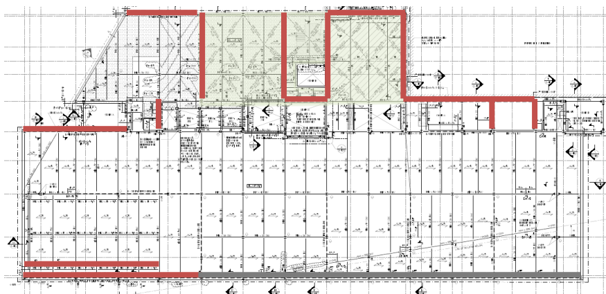
Figure 10: Level 5 Framing Plan Showing Lateral System (S-105) — Lateral Braced Frame — Gravity Truss that Contributes to Lateral System ■ Floor System with Diagonal Bracing
